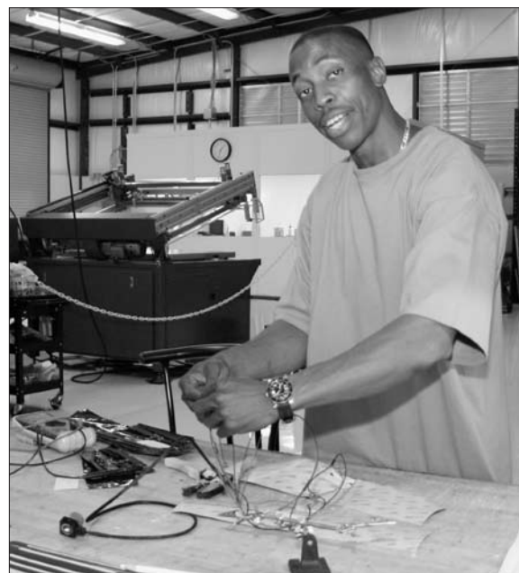
Johnny McKinney assembles wire harnesses for thermal wraps and attaches the thermostats.
